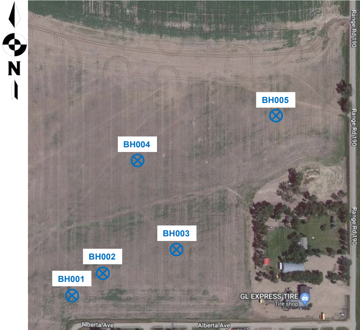
Figure 1 – Site Plan Borehole Location
