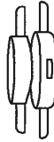
Long-handle double female swivel NST thread #225DF [specify size 2½-in.-6in. (63.5mm- 152mm)]
