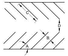
A: Parking Angle C: Depth Of Stall B: Width Of Stall
