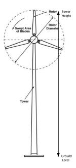
**Total Height** means the height from grade to the highest vertical extension of a SWECS. In the case of a SWECS with a horizontal axis rotor, total height includes the
