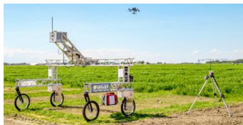
Fig.1 - Automated mobile robot (UFPS Cart) with GPS-GNSS RTK Base Station
