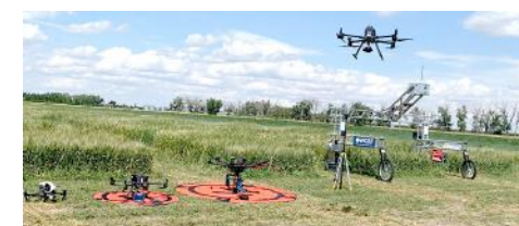
Fig.3 - UAV Imaging, UGV UFPS Cart, and D-RTK 2 GNSS Mobile Station
