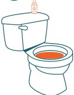
Return to the toilet where you placed colouring into the tank. Check the bowl of the toilet: is the water in the bowl clear or is there colour from the dye? If there is colour, water from the toilet tank is leaking into the toilet bowl. If the leak is large, you will be able to hear the toilet "running" and the dye will show up in the bowl
