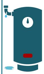
To inspect your boiler and hot water tank for leaks, look for water accumulation on the floor, or the tray under the unit.
