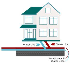
Water may be supplied to your home by a water line that is fed by a Main Water Line, located within the utility right-of-way, usually alongside the roads.
