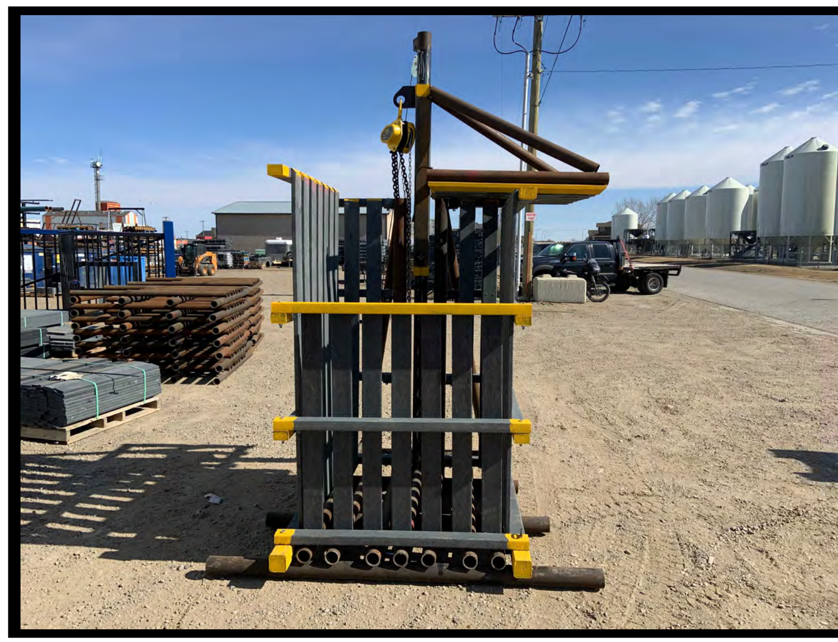
Ensure lid is in safety position and locked with safety pin before loading
