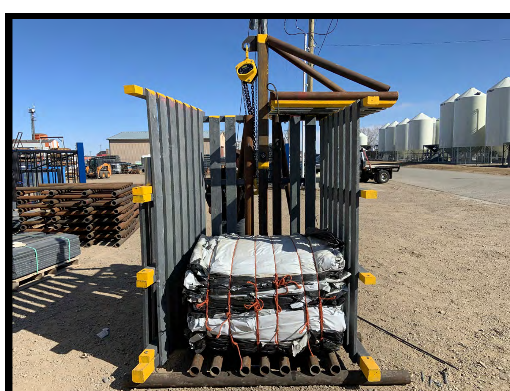
Raise lid & lock with safety pin
